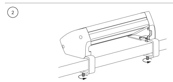
Attach unit by tightening screws to underside of table.
