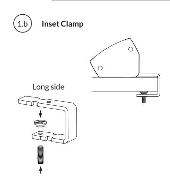
Insert long side of clamp into right and left end-caps.
