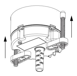
Tighten screws up against underside of desk/table top.
