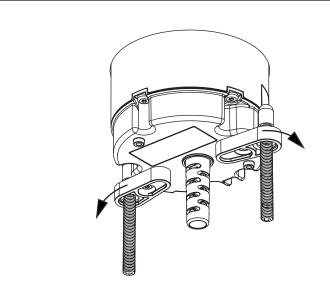
Once located in hole, swivel "wings" out until they've popped into position.
