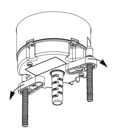
Once located in hole, swivel "wings" out until they've popped into position.
