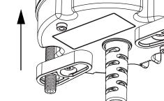
Tighten screws up against underside of desk/table top.
