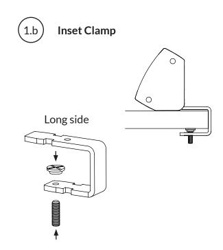
Insert long side of clamp into right and left end-caps.
