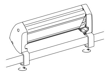
Attach unit by tightening screws to underside of table.
