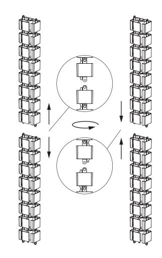
**Standard orientation:** rotate motion links 180° half way through spine length.
