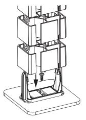
Attach bottom brackets to base using magnets and/or screw.
