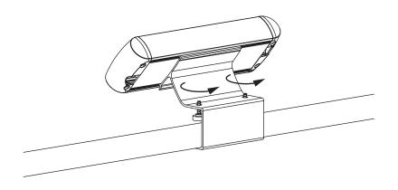
Attach unit by tightening screws securely against table, do not overtighten.
