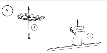
Attach top magnet clip by either screwing to surface or attaching using magnets.
