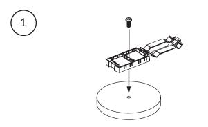
Attach Magnet to Base with Screws.
