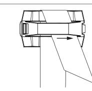
Pull Ribbon into notch to lock off.
