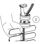
Bundle cables together. Close each link section around the cables.
