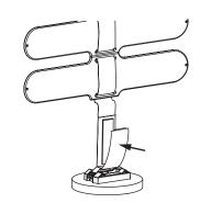
Attach Velcro loop through Magnet clip.
