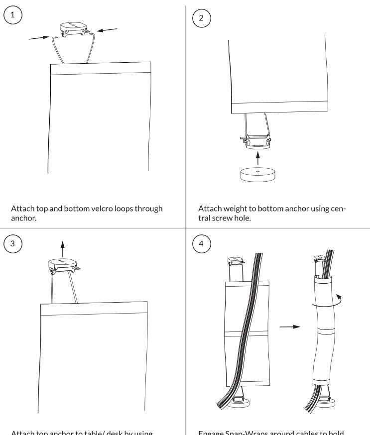
Attach top anchor to table/ desk by using either screw holes.
