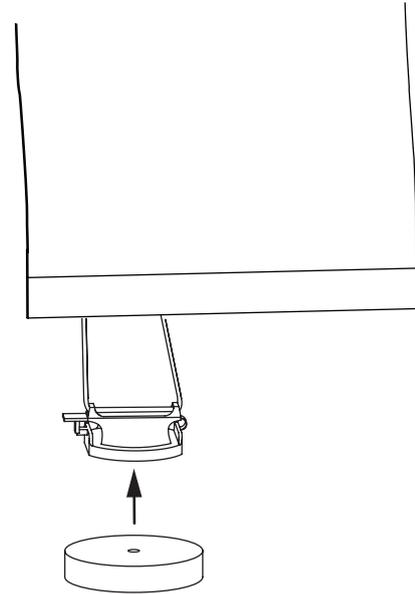
Attach weight to bottom anchor using central screw hole.
