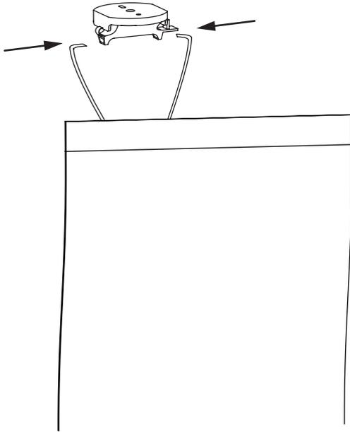
Attach top and bottom velcro loops through anchor.
