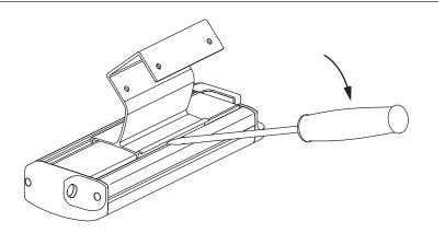
Attach unit by tightening screws securely against table, do not overtighten.
