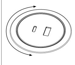
**5.3** Tighten screw wheel onto unit, sandwhiching the worktop.
