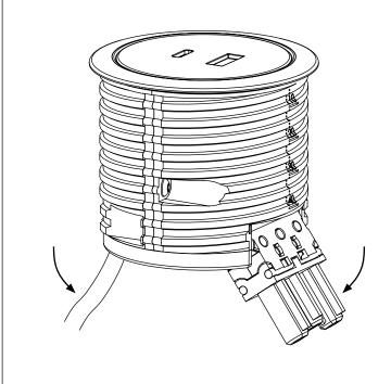
Place unit into pre-cut 60mm diameter hole in worktop.
