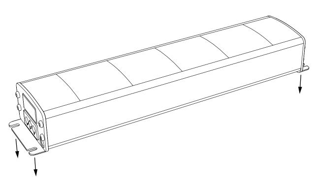
Attach unit to surface if needed via 4 alignment holes.
