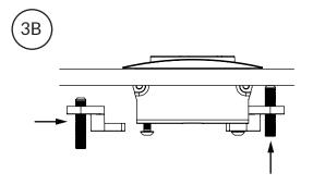
Attach brackets, tighten screws against table.
